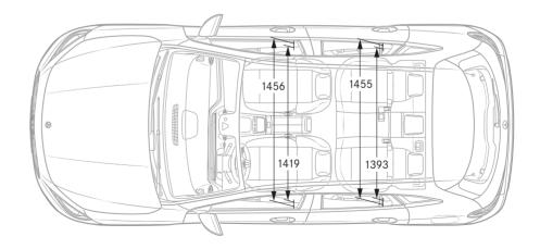
All figures in millimetres. The pictured dimensions are mean values. They are valid for vehicles with standard equipment and in unladen condition.
