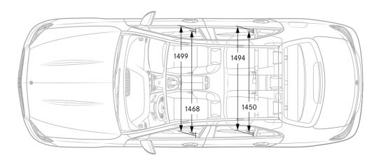
All figures in millimetres. The pictured dimensions are mean values. They are valid for vehicles in basic specification and in unladen condition.
